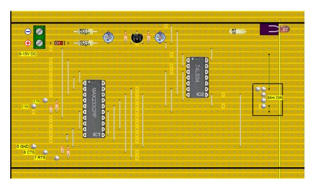
N.B. There are two links on the underside of the board from the mini din plug.
