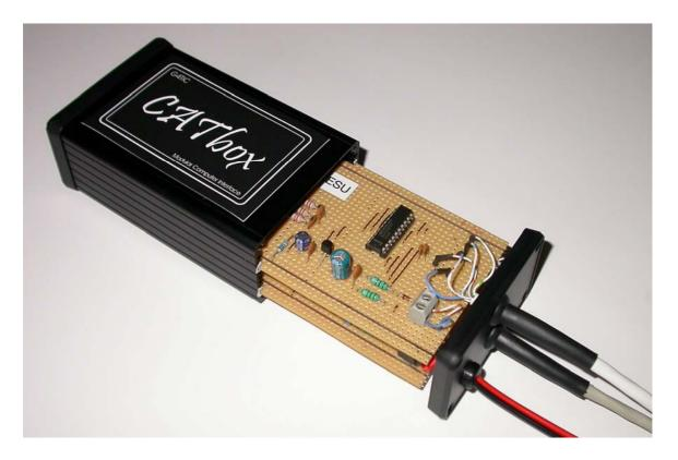
The screw connectors for the 12V supply allow easy interconnections between the two cards. The interconnecting wires are routed through conveniently sited holes in the matrix board from the lower to the upper card.
